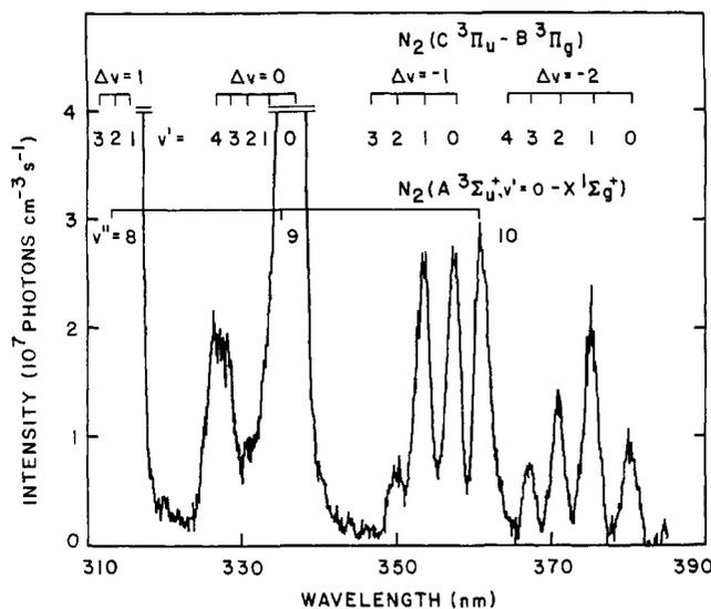
Figure 5. Vegard–Kaplan and second-positive bands (formed from  $N_2(A)$  energy pooling) in the presence of 3.5 mTorr of molecular oxygen.
