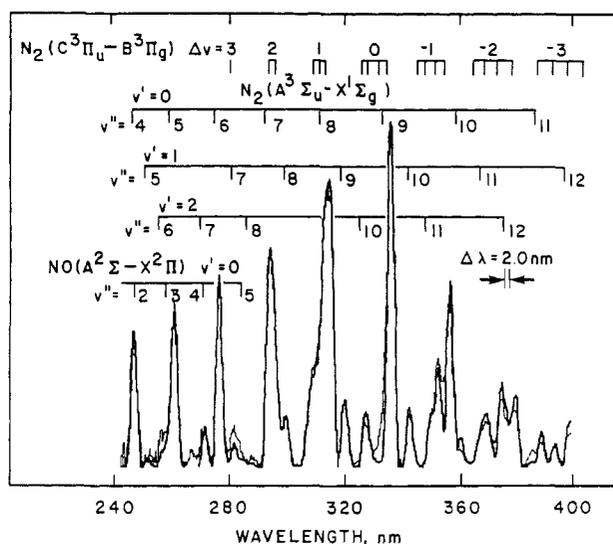
**Figure 1.** Data (light line) and best fit (dark line) to Vegard–Kaplan emission at 2.6 Torr. Included in the fit are first-positive emission, NO  $\gamma$  bands, and OH A–X emission (not shown) at 307 nm. The spectroscopic data have been obtained from the literature.<sup>17,23,24</sup>
