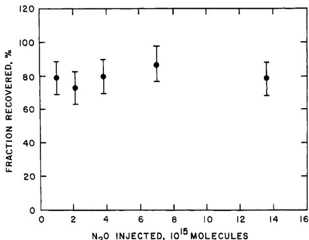
Figure 2.  $N_2O$  trapping efficiency. The data are presented as the fraction of  $N_2O$  recovered, in percent, versus the mass of  $N_2O$  injected.
